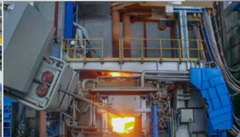
Electric Arc Furnace (EAF)
