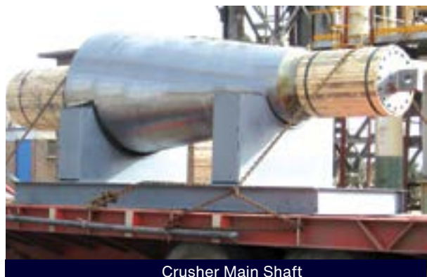
Crusher Main Shaft
